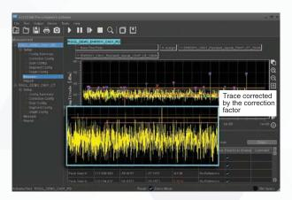
You can automatically load correction factors (preamplifier, attenuator, antenna, cable, or correction array) to carry out amplitude correction for the results
